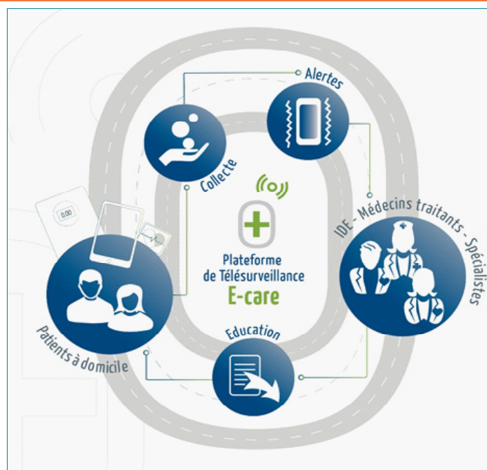
Figure 1. Version 1 of the generic telemedicine platform developed in the E-care project for remote monitoring of patients with heart failure. This platform is based on: non-intrusive medical sensors (TA, FC, O2, weight), communicating via Bluetooth, allowing to trace, in real time, physiological information on the state of health of the patient; a touch pad, communicating via Wi-Fi or 3G / 4G; and an Internet server hosting an inference engine generating alerts. These last ones sign a deterioration of the chronic pathologies of the patient. They are accessible to health professionals via a secure Internet portal.
